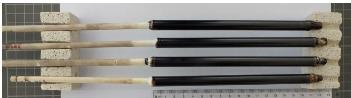
Figure 5. Thin composite-carbon membrane supported on porous alumina support.
