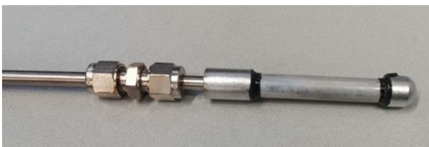
Figure 12. Membrane E722 sealed with two caps and black resin
